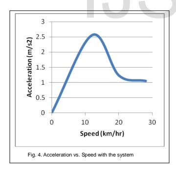
From the experiment findings, theoretical calculations and analysis of graphs, there is an evident acceleration boost when the proposed system is implemented. The acceleration boost percentage is approximately 9.3%.
